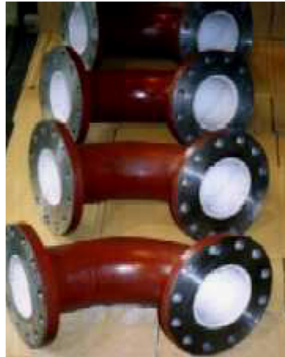
Fig. 4. Ceramic-lined tubes used for transferring powdery materials in the steel-making process. 10 Ceramic plates are bonded on the inner surfaces of steel tubes to improve wear resistance.
