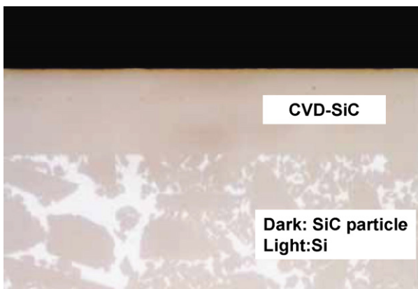
Fig. 2. A scanning electron micrograph of the cross-section of the SiC material. The material is reaction-sintered silicon carbide covered with dense CVD SiC on the surface. 7
